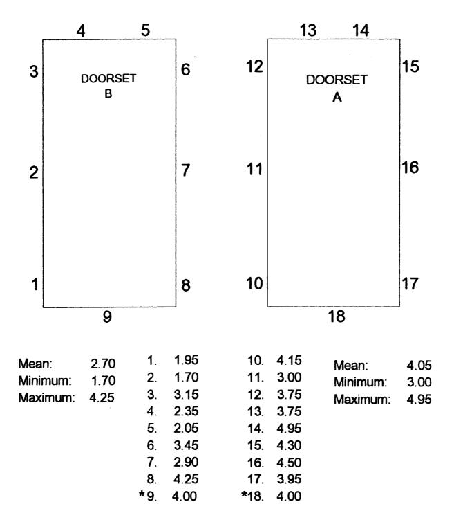
Dimensions measured between doors and frame as viewed from the exposed face. All dimensions in mm.
